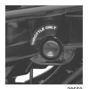
Throttle grip - Controls engine speed and shifting.
