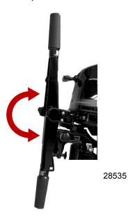
Tiller lock release lever - Push lever to move tiller handle from one position to another.
