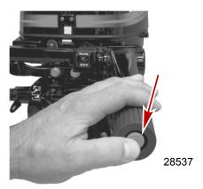
• Power tilt switch - Push to tilt engine up/down.
